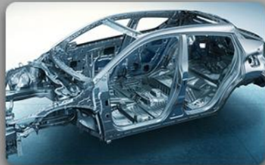
High-strength steel architecture
